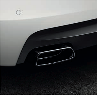
Tailpipes. The tailpipes on the left and right each come with a dark chrome trapezoid surround.
